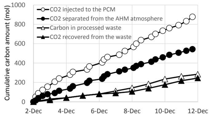
Fig. 3 Cumulative amount of carbon (mol) in CO<sub>2</sub> injected to the PCM, separated from the AHM atmosphere and recovered from the waste and carbon in processed waste from December 2 to December 11 in the last experiment conducted in 2007.
