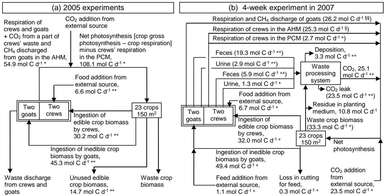
Fig. 2 A summary of carbon flows in 2005 experiments (a) and 4-week experiment in 2007 (b). \*: averages for three experiments in 2005, \*\*: averages for the last two experiments in 2005. †: averages for the last experiment in 2007. ++: averages for days without troubleshooting on waste processing system in the last experiment. Values in parentheses: estimated values. §: data in experiment without goats. §§: difference between data in experiments with and without goats.
