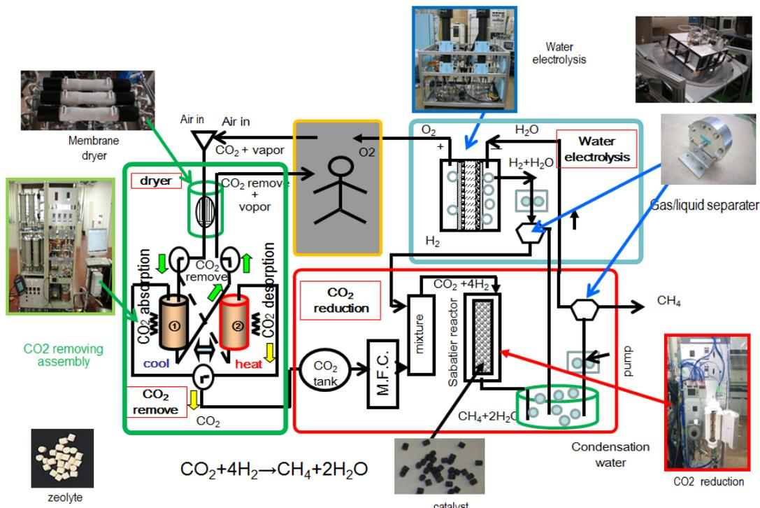
Figure 1 Concept of air revitalization system using CO<sub>2</sub> reduction
