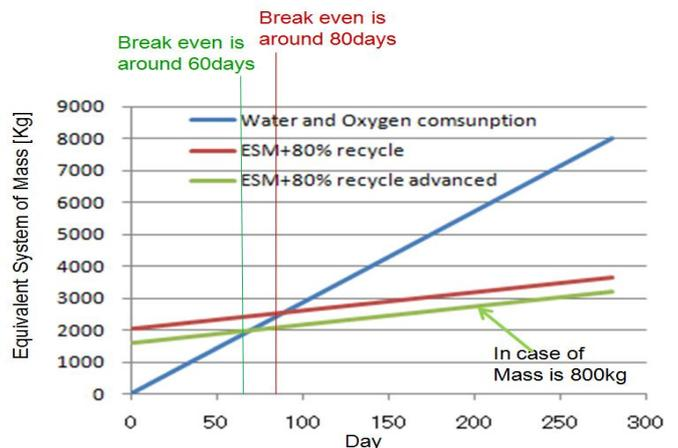
Figure 2 Breakeven point between non-regenerative ECLSS (pure consumption) and regenerative ECLSS
