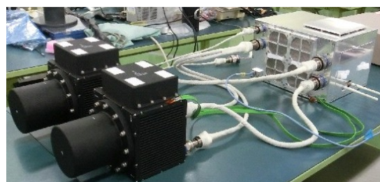
Fig.1 Photo of the PS-TEPC (flight model). The system consists of two detection parts (left, black color) and a control part (right, silver color). The cylindrical parts of the detection parts are the detection volumes of the PS-TEPC.
