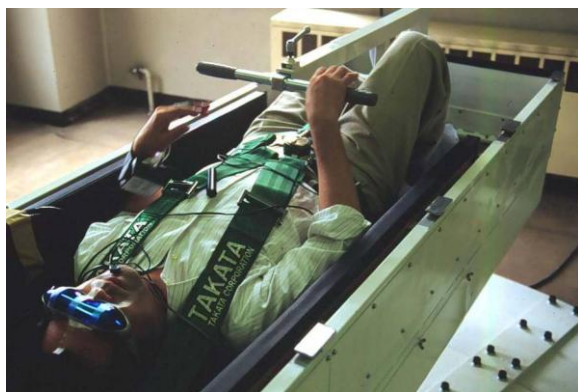
Fig.1 Manufacture of short radius centrifuge with lower leg ergometer.
