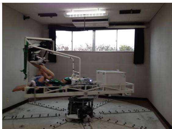
Fig.2 Manufacture of the remodeled short radius centrifuge with lower leg ergometer.
