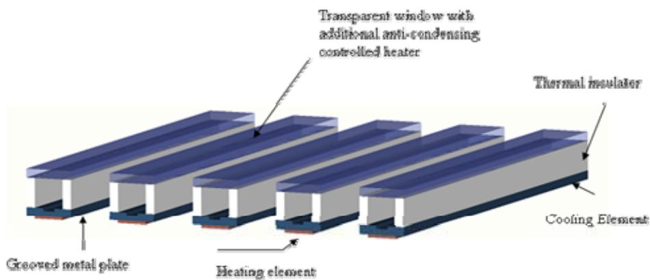
Figure 1: Typical layout with 5 model heat pipe cells
