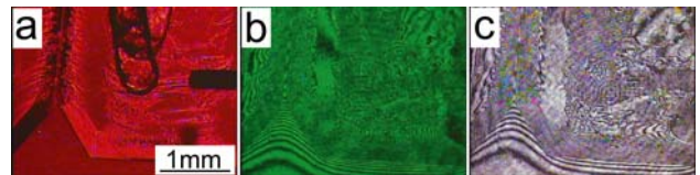
Fig. 4. Growing crystal at t = 7608\text{ s} under condition of temperature gradient of 7\text{K/cm} and cooling rate of 0.05\text{K/min} . The images are obtained by: (a) amplitude modulation microscope, (b) 532-nm interferometer, (c) 780-nm interferometer.
