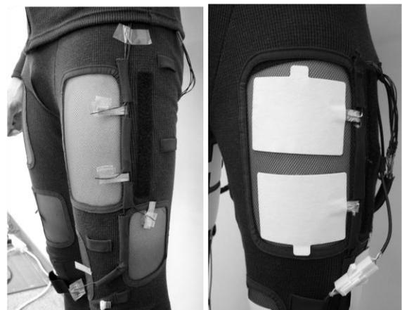
Fig.3: Electrodes position of the device. The suit was made with partly electric conductive meshes covering the motor points, which were designed to attach the electrodes (Sekisui Plastics, Tokyo Japan) onto them and stimulate the muscles adequately.
