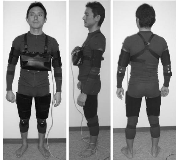
Fig.2: Wearable device to maintain skeletal muscles in space by utilizing HYB system. The electric wires and joint motion sensors were also attached in the suits (Goldwin inc. Tokyo, Japan).
