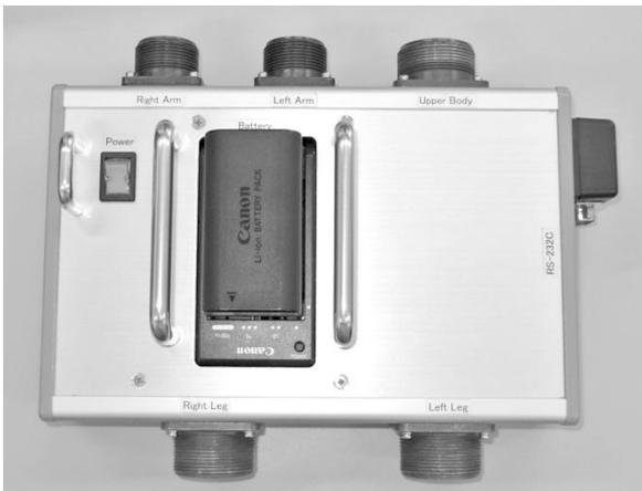
Fig.4: Stimulator and battery. Its size was 220mm in length, 140mm in width, and 55mm in height, and weight was 1,030g (Logical Product Inc., Fukuoka, Japan).
