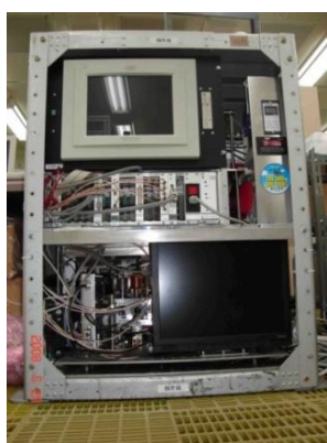
Fig.1 PK-3 Plus experimental model installed in a rack for parabolic flight.
