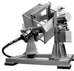
Fig. 1. Photograph of the 3D-clinostat. By controlled simultaneous rotation of two axes, the 3D-clinostat cancels the cumulative gravity vector at the center around the device, producing an environment with an average of 10^{-3} G over time.
