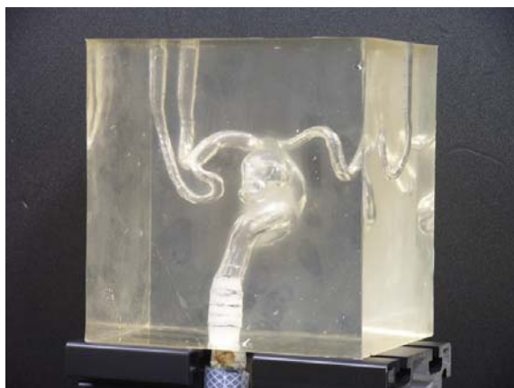
Fig.2 Silicone model of cerebral artery.
