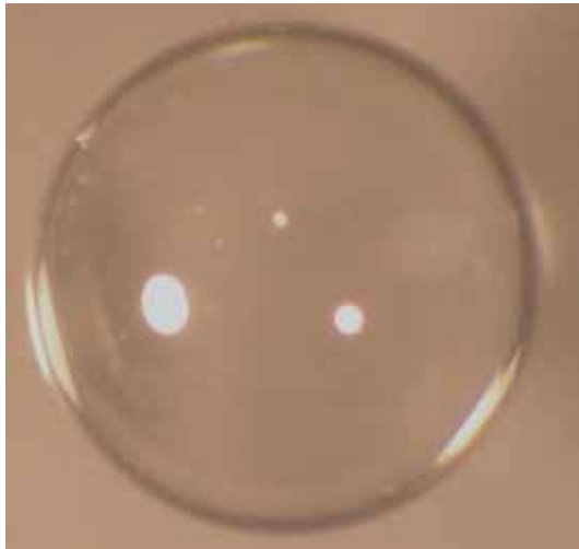
Figure 3. Morphology of BaTi 2 O 5 glass fabricated by containerless processing
