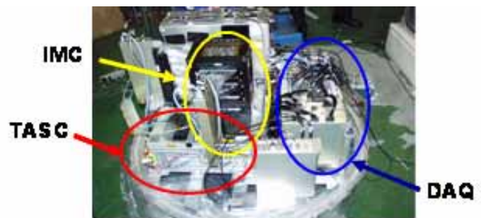
Fig. 1 CALET proto-type for balloon experiment. It is composed of Imaging Calorimeter (IMC) and Total Absorption Calorimeter(TASC), and Data Acquisition System (DAQ). The scale of detector is nearly 1/64 in size and the weight is about 250kg.
