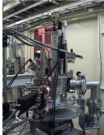
Fig.2 An electrostatic levitator combined with X-ray
