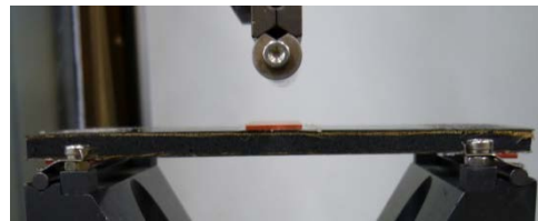
Fig. 4 Test configuration for three-point bending test.
