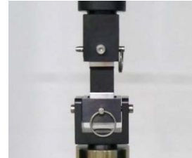
Fig. 3 Test configuration for flatwise tensile test.
