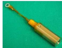
Fig. 6 Exterior of PPT head
