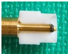
Fig. 5 Cross section of propellant and anode after 10,000-shot operation (Energy density:  $0.23 \text{ J/mm}^2$ )
