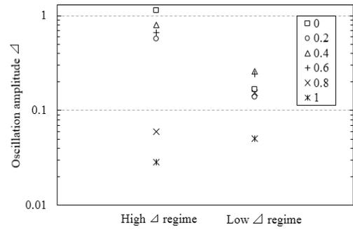
Figure 1 As the  $\dot{m}_{diff}/\dot{m}_{tot}$  increases, discharge oscillation is being suppressed in both regimes.
