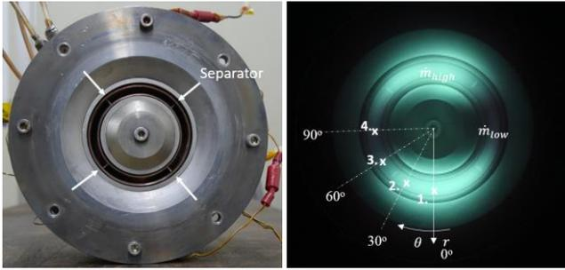
(a) Anode layer thruster R66 (b) local measuring positions
