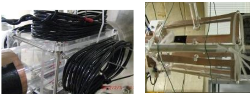
Fig. 3 RMF coils: (a)10 turn, (b)1 turn
