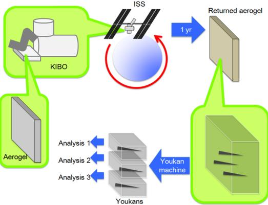
Fig. 1 A schematic illustration of the Tanpopo mission.
