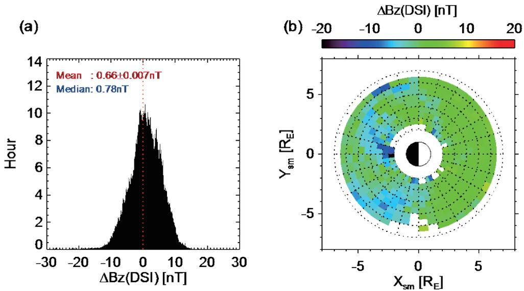
Fig. 1 (a) Histogram of the  $\Delta B_{z, \text{DSI}}$  with a 0.1 nT bin. (b) Distribution of the  $\Delta B_{z, \text{DSI}}$  projected onto the R-MLT plane in SM coordinates. Each mesh size is 0.5 hr MLT by 0.5  $R_E$ .
