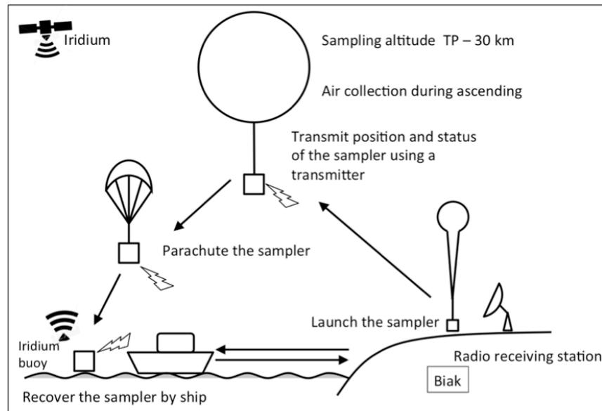
Fig. 1. Schematic diagram of stratospheric air sampling.
