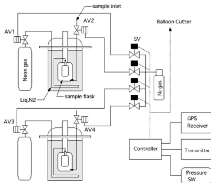
Fig. 2. Schematic diagram of the balloon-borne air sampling system. SV and AV mean solenoid valve and pneumatic valve, respectively. A sample flask is set in a dewar filled with liquid nitrogen. The J-T mini cooler is fixed in the sample flask.
