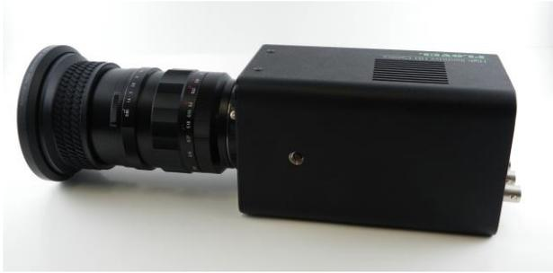
Fig. 1. Photo of (a) the HbCMOS HDTV camera attached with a lens and a wide-angle converter, (b) WORF rack in Destiny (Photo courtesy NASA). Observation is done through the window.
