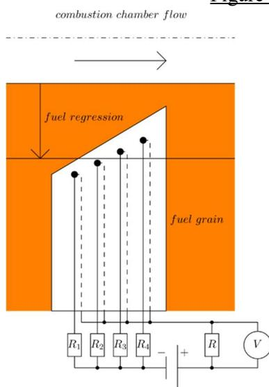
The RBS developed by Politecnico di Milano are based on the same principle but with a different architecture: the resistors themselves are located outside of the grain. The regression of the sensor's raw material conducts to the disconnection of the resistors and hence to the variation of the output electric voltage (Fig. 3).
