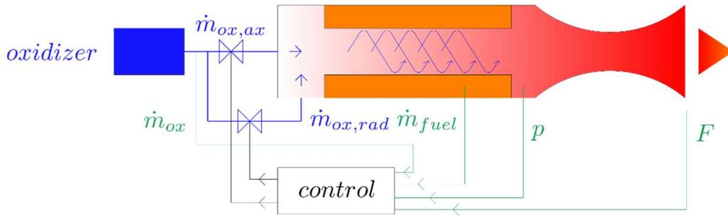
Figure 1. A-SOFT engine concept and its feedback loop control.
