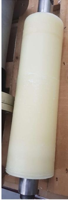
Figure 5. Wax-fuel grain manufacturing process.
