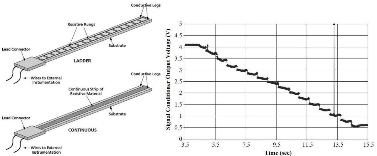
Figure 2. MIRRAS sensors (left) and signal (right).
