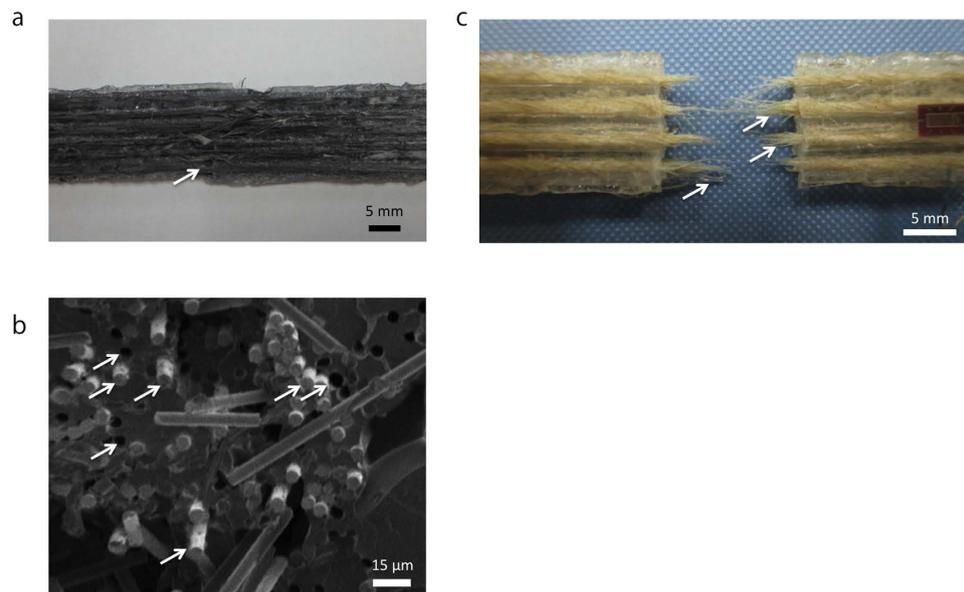
**Figure 5. Fracture of a unidirectional continuous FRTP fabricated by 3D printing.** Fiber pullout due to tensile fracture observed as an (a) overview and (b) scanning electron microscopy image of the CFRTTP specimen. (c) Fiber pullout in the JFRTP specimen.
