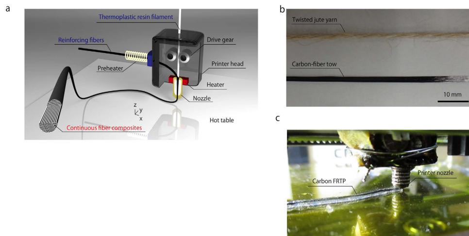
**Figure 1.** (a) Schematic of the 3D printer head used to produce continuous FRTPs using in-nozzle impregnation based on FDM. (b) Continuous fiber reinforcements used for 3D printing. (c) Photograph of the 3D printing of a CFRTF.
