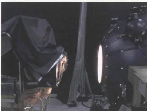
Fig. 2 Radiometric performance test of the LISM using the 1 m \phi integrating sphere.
