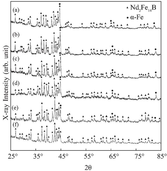
Fig. 3 XRD pattern of the  $\text{Nd}_2\text{Fe}_{14}\text{B}$  alloy ingots (a) and (b), (c), (d), (e), and (f) depict the profiles of samples with 2000  $\mu\text{m}$ , 500  $\mu\text{m}$ , 400  $\mu\text{m}$ , 350  $\mu\text{m}$ , and 250  $\mu\text{m}$ , respectively.
