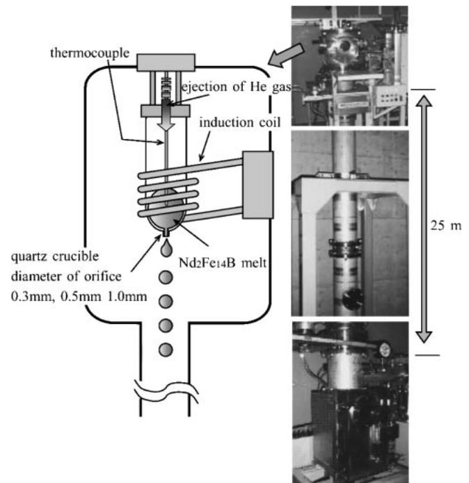
Fig. 1 Schematic diagram of the drop tube experiment.
