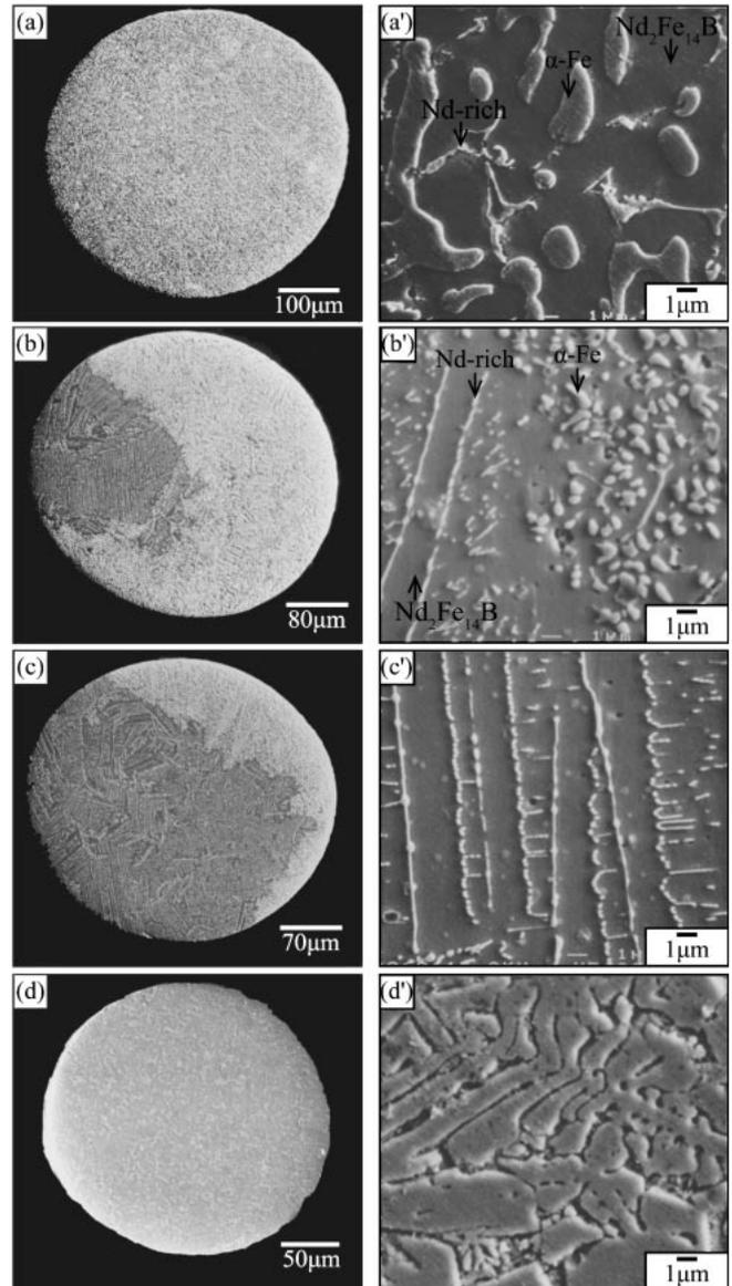
Fig. 4 Cross sectional microstructures of  $\text{Nd}_2\text{Fe}_{14}\text{B}$  alloy with (a) 500  $\mu\text{m}$ , (b) 400  $\mu\text{m}$ , (c) 350  $\mu\text{m}$ , and (d) 250  $\mu\text{m}$  in diameter. (a'), (b'), (c') and (d') are further magnified microstructures of those at the center, respectively.
