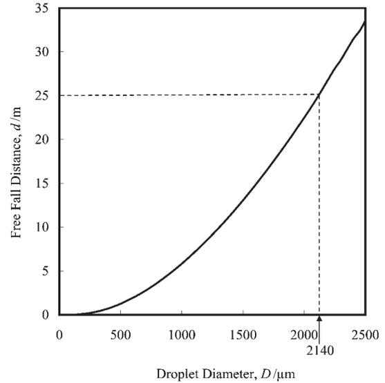
Fig. 2 Free fall distance as a function of the sample diameter.
