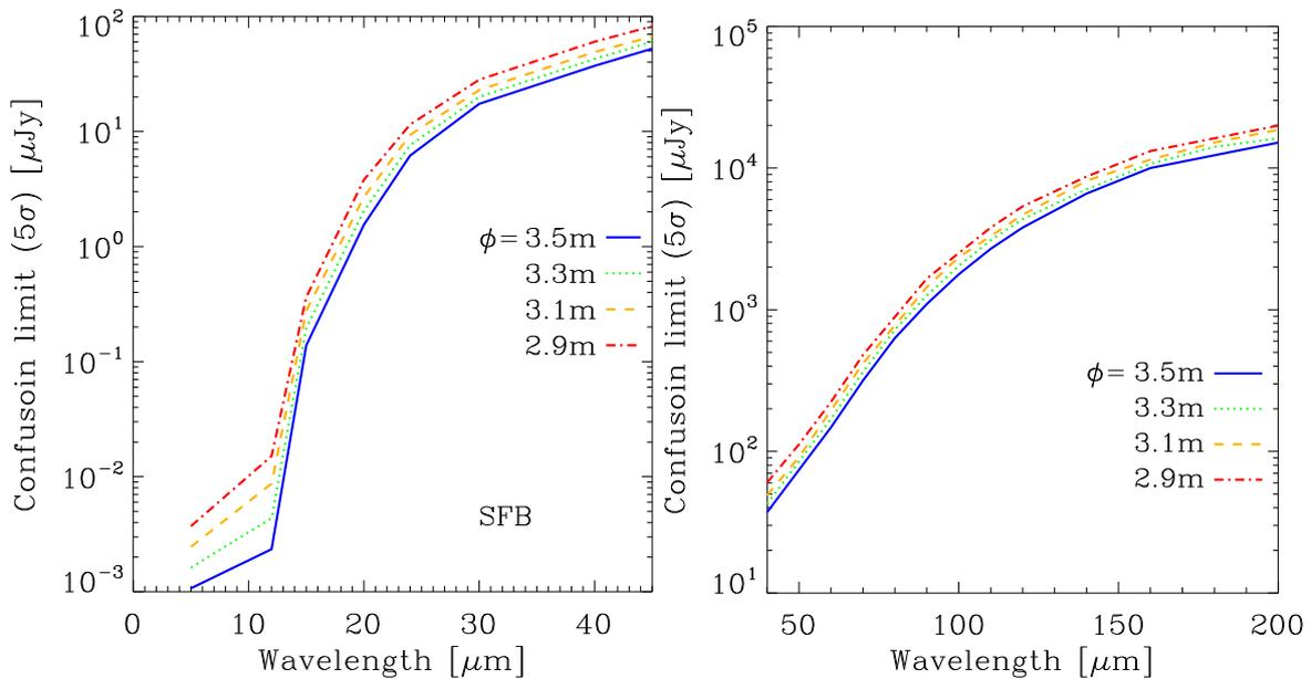
**Figure 3.** The *SPICA* confusion limits as a function of the mirror diameter. Left-hand panel shows the confusion limits at the MIR wavelengths, and right-hand panel shows the limits at the FIR wavelengths.
