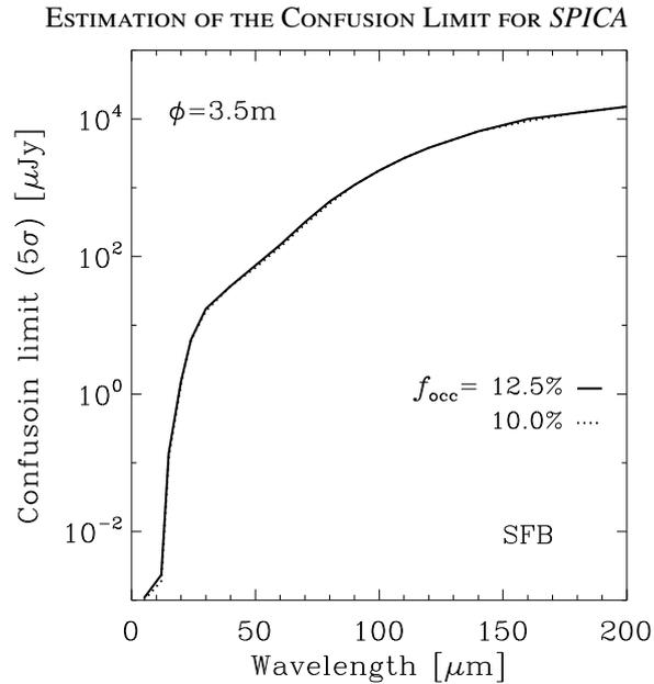
**Figure 2.** The confusion limit expected for *SPICA*. Results for the occultation fraction  $f_{\text{occ}} = 0.1$  (goal: dotted line) and 0.125 (worst: solid line) are presented.
