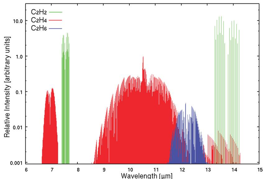
**Figure 2.** The synthesized spectra of the hydrocarbon molecules that have fundamental vibrational transitions around 10 μm region. We expect strong fluorescence emission lines of C<sub>2</sub>H<sub>2</sub>, C<sub>2</sub>H<sub>4</sub> and C<sub>2</sub>H<sub>6</sub> in this wavelength region. C<sub>2</sub>H<sub>4</sub> has especially strong emission bands while this molecule has never been detected in comets in the near-infrared wavelength region.
