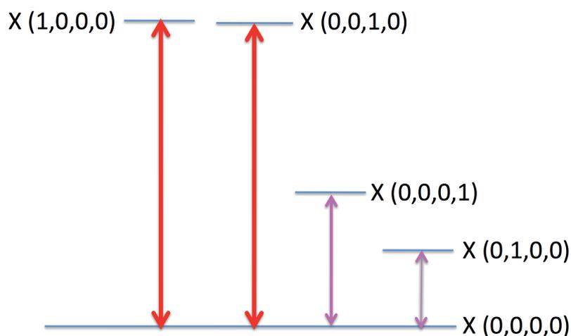
**Figure 1.** Fluorescence excitation model of NH<sub>3</sub> as an example. The fluorescence excitation model of each molecular species includes its fundamental transition. The solar radiation field is considered as the main energy source for pumping from the ground state.
