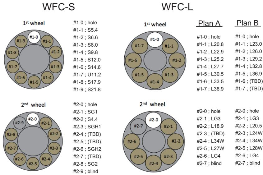
**Figure 1.** Available slots for filters and grisms for WFC-S and WFC-L.**5. TECHNICAL CONSTRAINTS FOR THE CHOICE OF FILTERS AND GRISMS FOR WFC**
