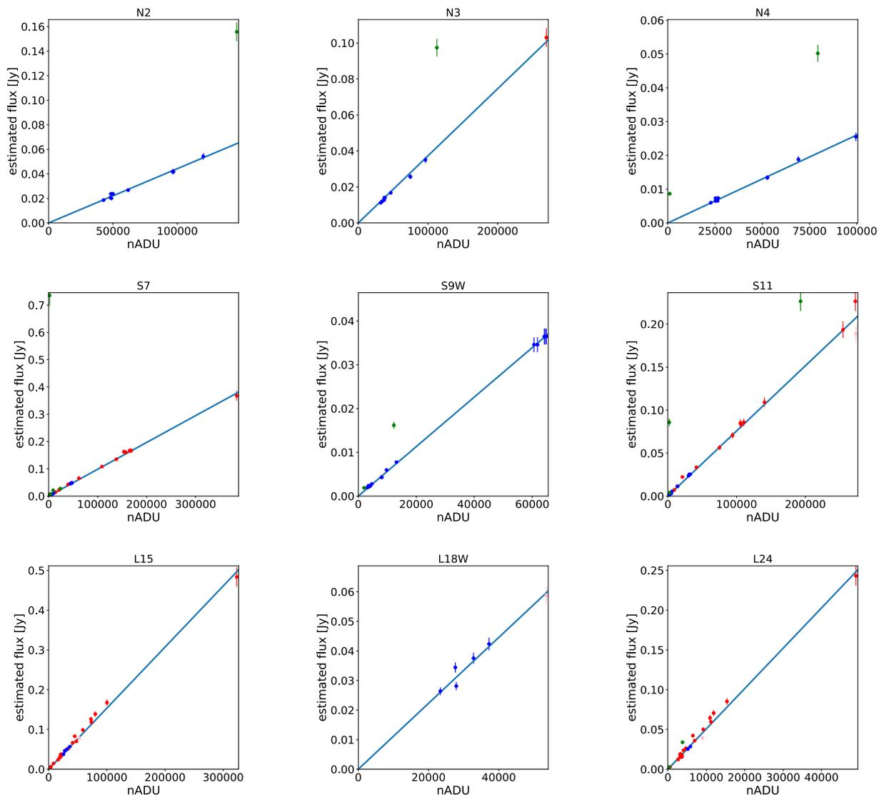
**Figure 1.** Relationship between the estimated flux (Jy) and the observed data values (nADU). Dots denote standard stars. (Blue, red and pink are stars in LMC, NEP and SEP, respectively.) Blue line is a least-square fit to the data (except for the green dots, which were excluded from the fitting).
