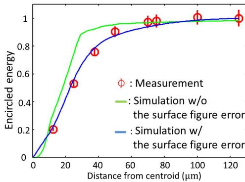
**Figure 3.** Encircled energies obtained by the optical testing and simulations. Red points show the measurement results, while blue and green lines show the simulation results with and without the surface figure error of the camera lens, respectively.
