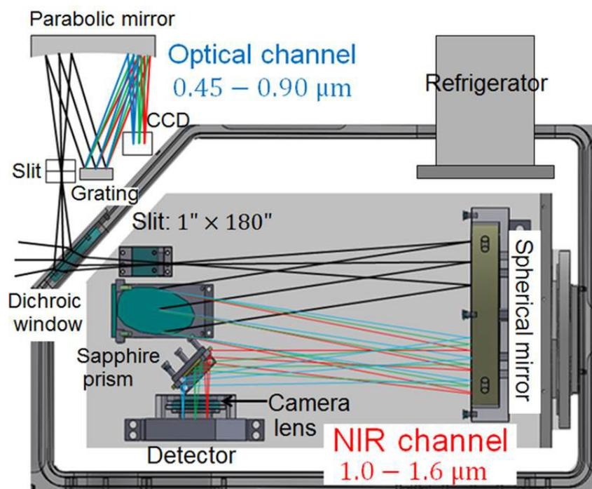
**Figure 1.** Optical layout of the NIR and optical spectrometer for the IRSF telescope.
