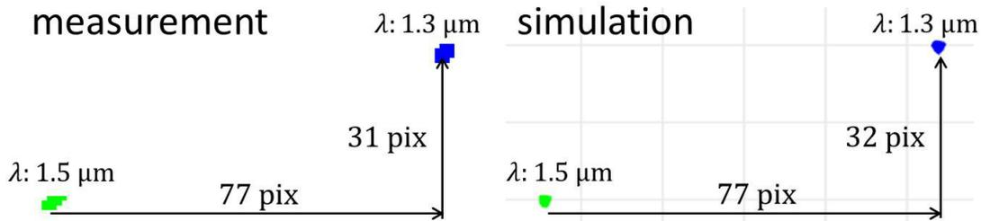
**Figure 2.** Measured and designed focus positions on the detector array at wavelengths of  $1.3 \mu\text{m}$  (blue) and  $1.5 \mu\text{m}$  (green). Arrows show the distances on the pixel scale.
