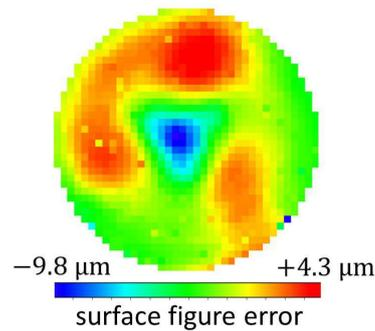
**Figure 4.** Measured surface figure error of the camera lens. Color bar shows the surface figure error in units of  $\mu\text{m}$ .
