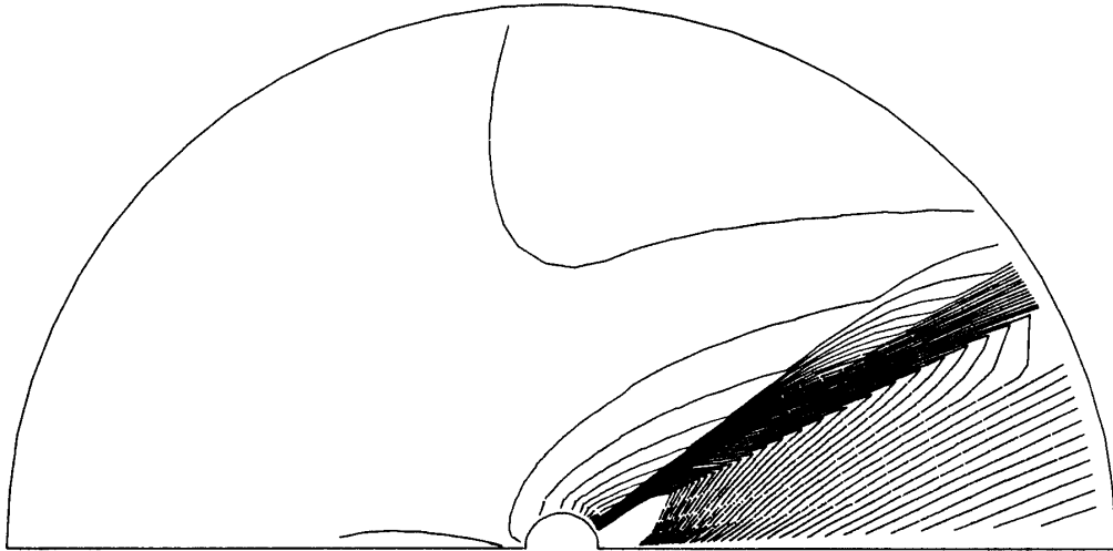
Fig. 7. Density distribution of the flow interacting with a absorbing gravitating sphere. An accretion radius is four times of the radius of the sphere. An intense accretion shock is formed. The maximum of the density occurs at the back side of the sphere. Other nomenclator are the same as Fig. 6.
