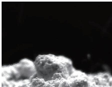
Fig. 4. Silica dust lofting under the electron beam.
