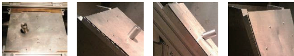
90deg_Penetrating Metal Anchor 1, 60deg_Penetrating Metal Anchor 1, 45deg_Penetrating Metal Anchor 2, 30deg_Sliding Metal Anchor 2
