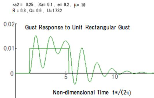
Figure 3: Transient response of the aeroelastic system
