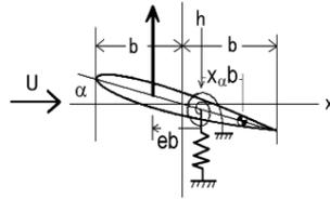
Figure 1: Typical Section Airfoil
