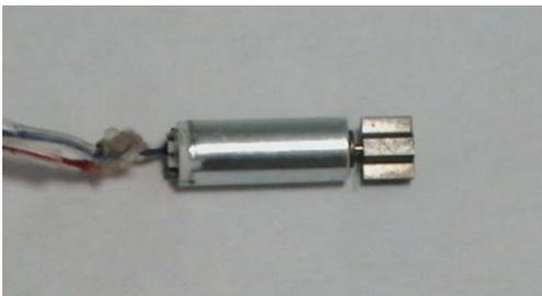
Photograph 1. Micro vibration motor.
