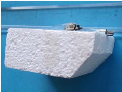
Photograph 8. Surface tension wave making propulsor. Model advancing direction is right of the photo.
