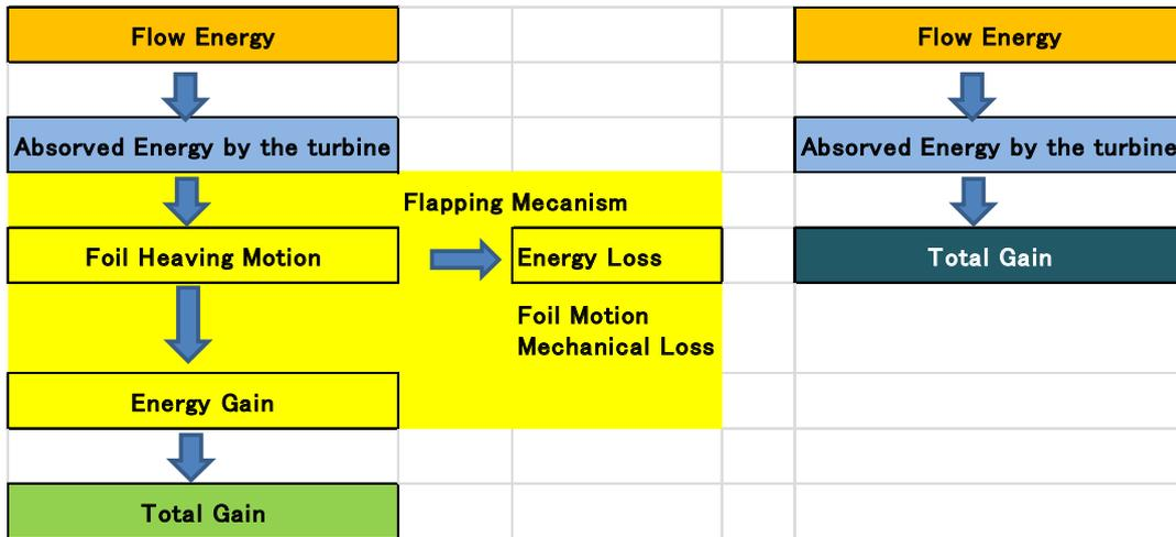
Figure 5. Energy flow diagram (left is FVAWT and right is fixed pitch normal VAWT)
