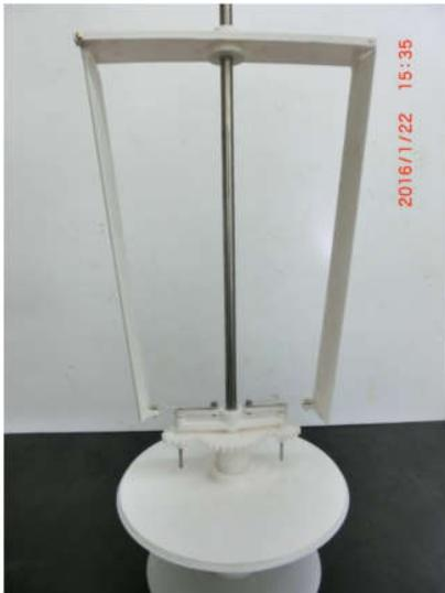
Photograph 1. Foil Closed FVAWT with spur gear.
