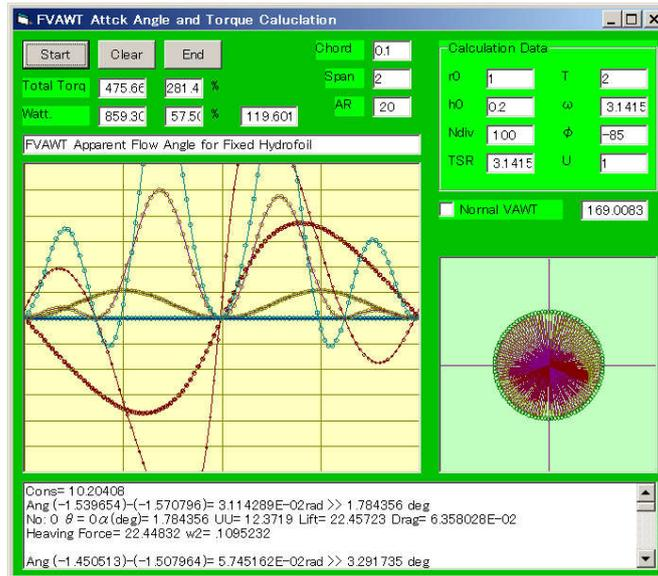
Figure 6. A sample of the FVAWT calculation.
