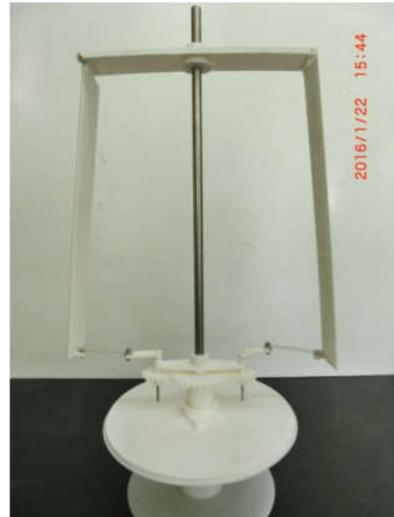
Photograph 2. Foil Opened FVAWT with spur gear.
