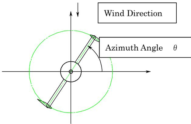
Figure 3. Normal VAWT at operation.
