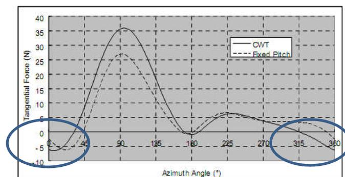
Figure 1. VAWT hydrofoil thrust (tangential) force.
