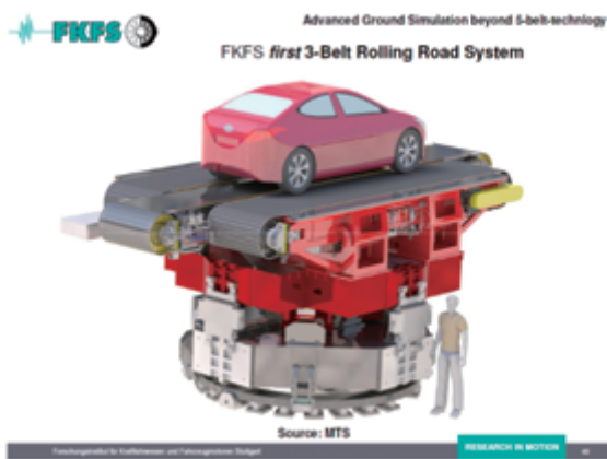
Fig 4 3-belt System of Future FKFS Wind Tunnel
