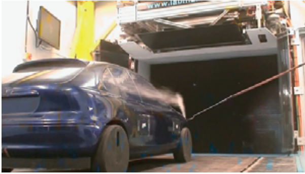
Fig 6 40% Scale Wind Tunnel with Flaps of Durham University
