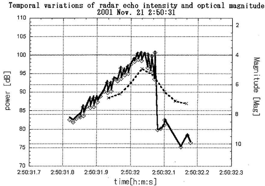
Fig. 3: Time variation of radar echo intensity and optical magnitude of the meteor observed at  $2^h50^m31^s$  JST on November 21, 2001. The open diamond shows observed echo intensity. The solid line shows the radar echo intensity with the antenna gain pattern corrected. The dotted line is absolute magnitude observed by the ICCD camera.
