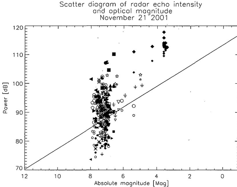
Fig. 5: Scatter diagram of instantaneous (1/30 sec average) radar echo intensity and optical magnitude. The data for the same meteors are plotted with the same symbols. The small symbols show observed echo intensity. The large symbols show the radar echo intensity with the antenna gain pattern corrected. Data with beam pattern correction larger than 30 dB are removed. The solid line indicates the relation obtained by Nishimura et al. (2001).
