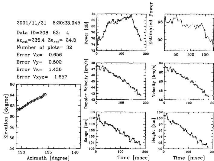
Fig. 2: An example of the radar observation result. The left panel shows tracks of the meteor head in apparent directions observed by the radar. Observed radar echo intensities (antenna gain pattern uncorrected), Doppler velocities, ranges are displayed in the center column (from the top to the bottom). Similarly, radar echo intensities with antenna gain pattern corrected, meteor head velocities, and heights are plotted in the right column.
