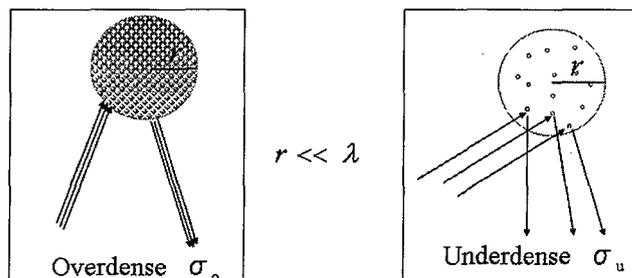
Fig. 6: Simplified model of radio scattering for overdense (left) and underdense (right) head echoes. Note that the radius of the meteor head,  $r$ , is assumed to be much smaller than the radar wave length,  $\lambda$ .
