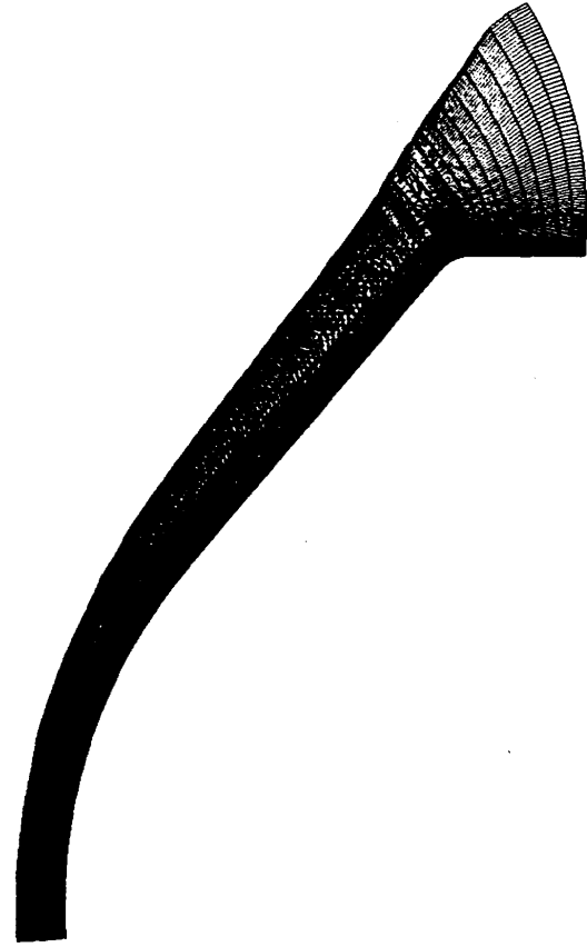
Figure 1: An example of body-oriented grid system. \xi \times \eta = 51 \times 150
