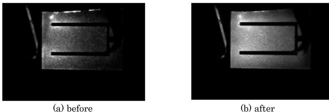
**Figure 2.** EL images of CIGS solar cells (a) before and (b) after electron irradiation at 120 K. The electron fluence was  $3 \times 10^{15} \text{ cm}^{-2}$ .
