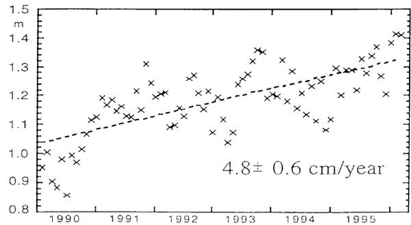
Fig. 7a. Time-dependent height difference between the tide gauge stations Kozu-Jima and Minami-Izu
