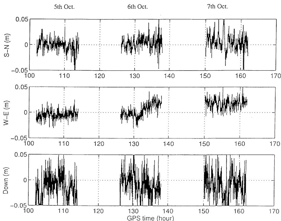
Fig.9. Change of the baseline vector from Kozu-Jima to Nii-Jima before and after the Earthquake on 6th Oct. '95 calculated by Kinematic GPS
