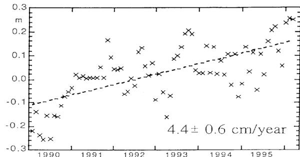
Fig. 7c. Time-dependent height difference between the tide gauge stations Kozu-Jima and Shimizu-minato
