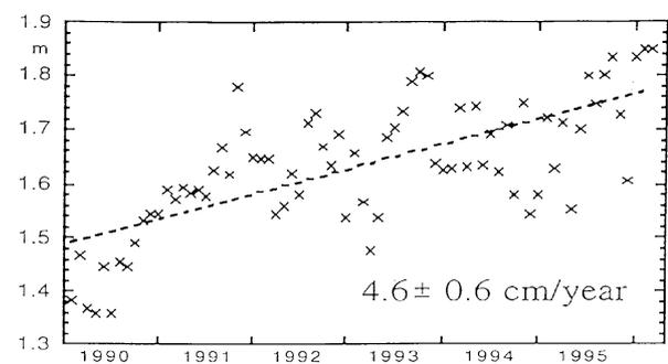
Fig. 7b. Time-dependent height difference between the tide gauge stations Kozu-Jima and Yaizu
