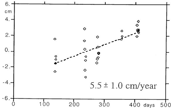
Fig. 3. Height difference between Kozu-Jima and Shizuoka estimated by GPS
