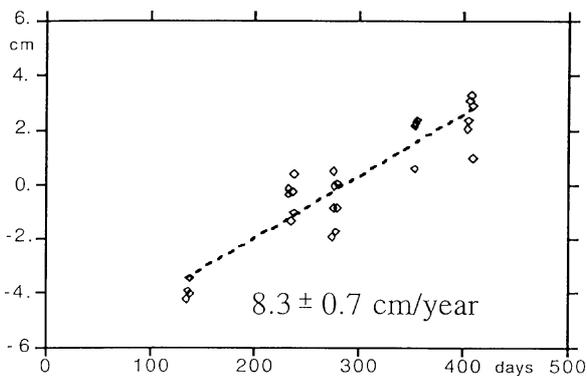
Fig. 1. Height difference between Kozu-Jima and Shizuoka estimated by GPS
