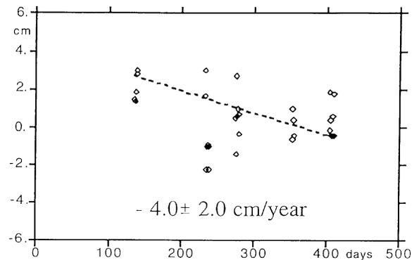
Fig. 5. Height difference between Shizuoka and Usuda estimated by GPS
