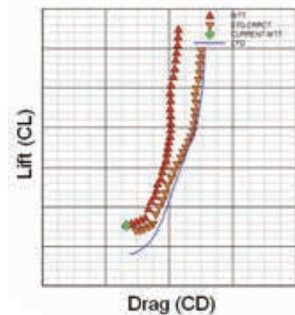
(c) Drag polar plots (comparison between WT data with/without support interference correction).
