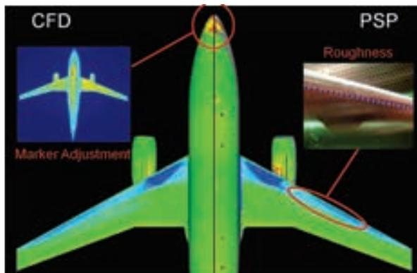
(d) Comparison of pressure distribution by EFD (PSP) and CFD and error sources of PSP measurement.
