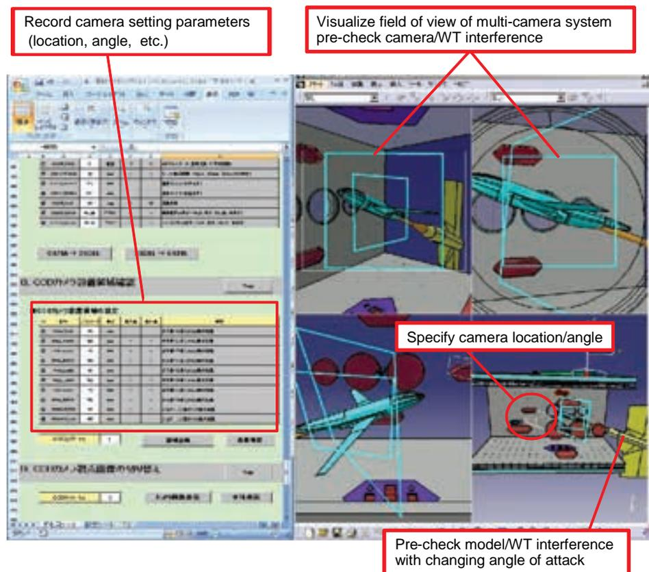
Figure 4 CAD-based wind tunnel test setting simulation.
