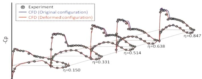
(c) Comparison of chord-wise static pressure distribution at five spanwise locations on the main wing.
