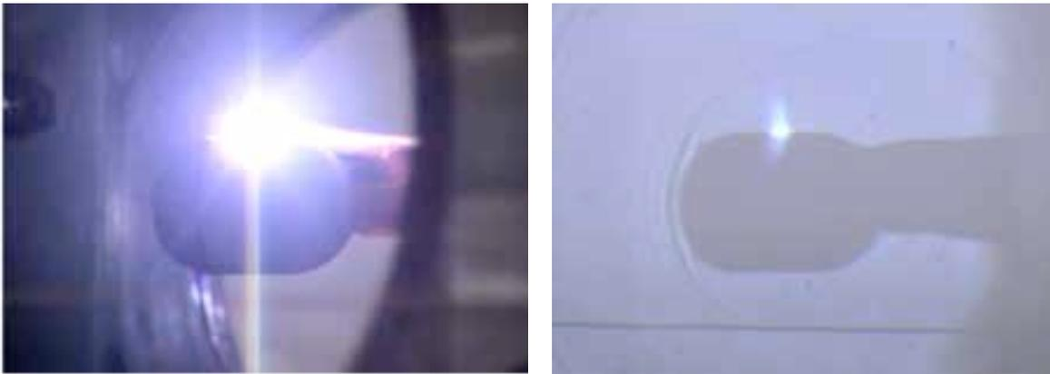
**Fig. 10 Snapshots of Normal Video (left) and Schlieren Video (right) of Model in Hypersonic Flow with Electric Discharge**
