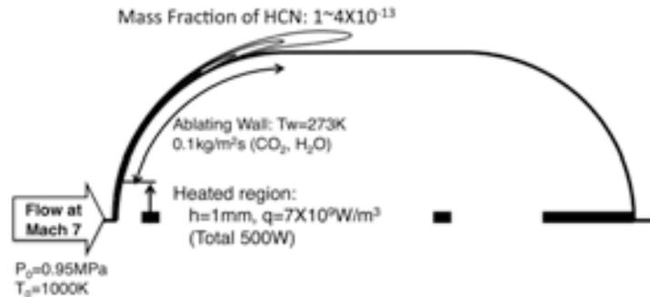
Fig. 8 Mass Fraction of HCN by CFD in Case of Electric Discharge in Stagnation Region
