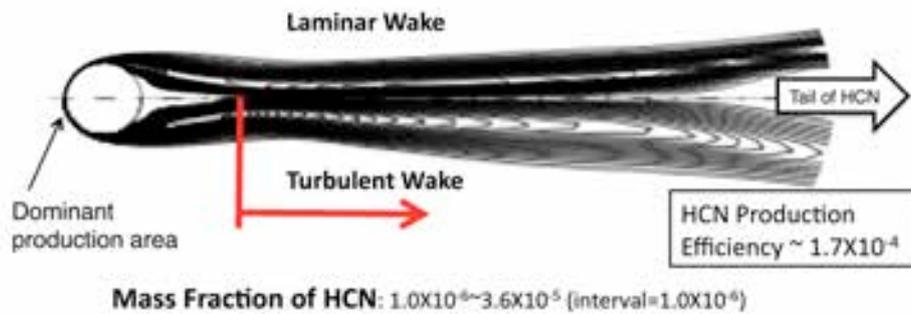
Fig. 3 Typical CFD Result on HCN Production
