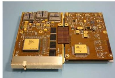
Fig. 11. The TDM Flight Unit folded out.
