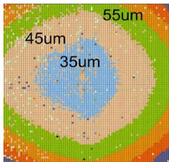
Fig. 6. Back-side thinned DDR-II memory – thickness in um.
