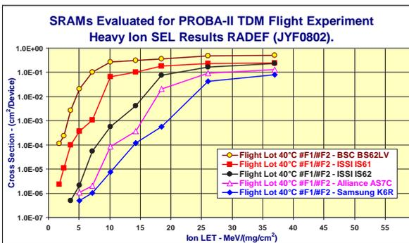
Fig. 13. SRAMs Latch-up sensitivities at 40 °C.
