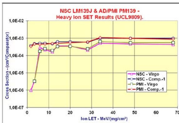
Fig. 17, NSC and PMI 139 Heavy ion SET results.
