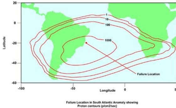
Fig. 14, ERS-1/PRARE Failure location, proton latch-up.
