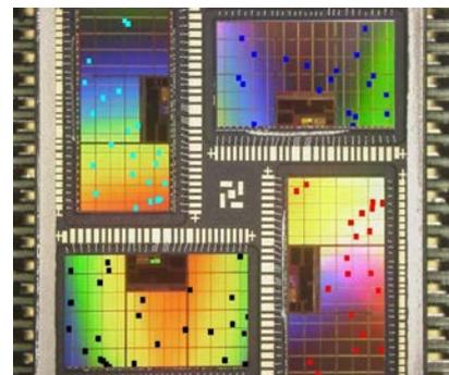
Fig. 10. SEU in the new detector element, the AT68166 MCM.
