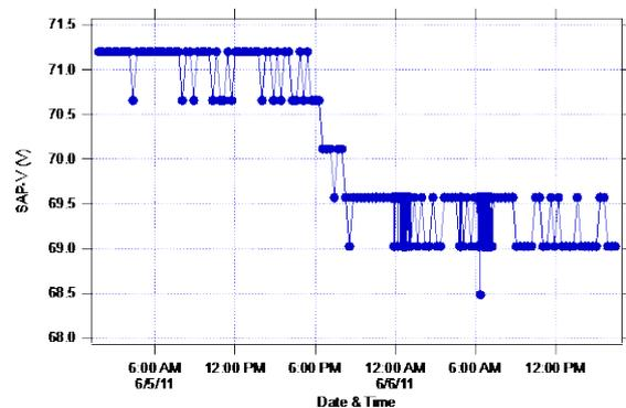
Fig. 3 Solar array output voltage trend showing sudden voltage drop on June 5, 2011.
