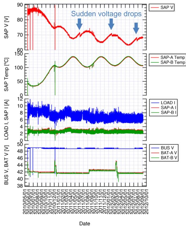
Fig. 2 Solar array-related telemetry data since launch.
