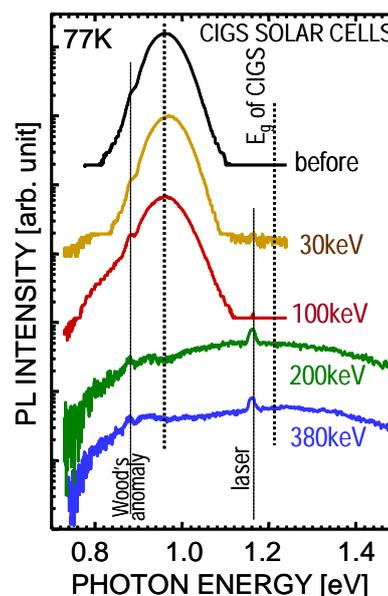
Fig. 4. PL spectra of CIGS solar cells at 77 K irradiated with  $3 \times 10^{15} \text{ cm}^{-2}$  as a function of proton energy.
