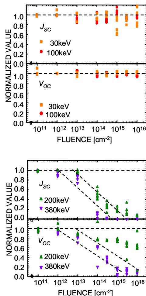
Fig. 5. The normalized (a)  $J_{SC}$  and (b)  $V_{OC}$  values of CIGS solar cells irradiated with 30 and 100 keV and (c)  $J_{SC}$  and (d)  $V_{OC}$  values of CIGS solar cells irradiated with 200 and 380 keV as a function of proton irradiation fluence.
