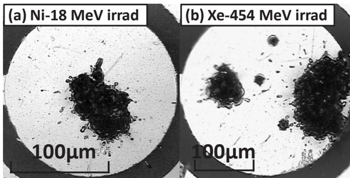
Fig. 2: Optical microscope images of electrode in MOS capacitor irradiated with Ni-18 MeV and Xe-454 MeV.
