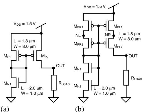
Fig. 3. Current mirror circuit without RHBD (a), and Current mirror circuit with RHBD (b). Output current set to 100 nA for both circuits at  $V_{DD} = 1.5 \text{ V}$ .
