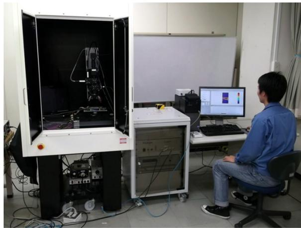
Fig.3. Pulsed-laser SEE test system. (@ JAXA Tsukuba Space Center.)
