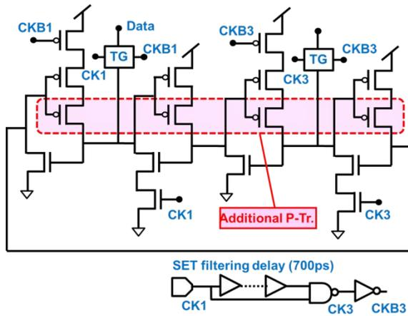
Fig.1. Schematic diagram of modified DICE.
