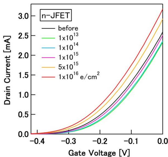
Fig. 2. Input characteristics of the n-JFETs before and after the electron irradiation.
