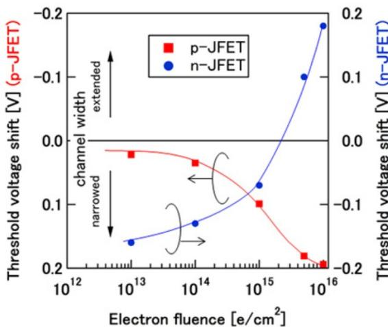
Fig. 4. Shift of  $V_{TH}$  by electron irradiation for p- and n-JFETs.
