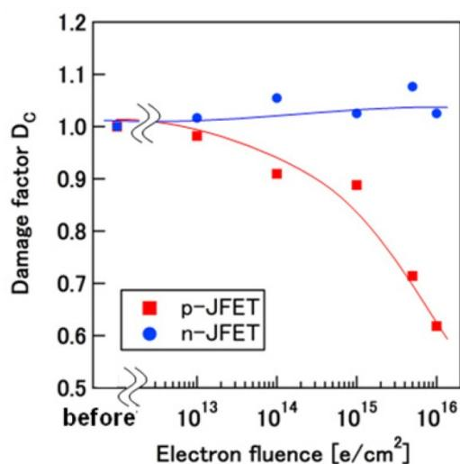
Fig. 5. The damage factor of carrier density ( $D_C$ ) for the p- and n-channel after the electron irradiation.
